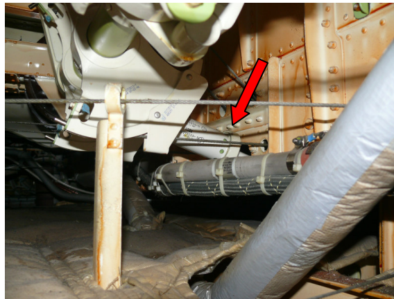
Photo 15. Load Limiter of the nose alternate landing gear extension system.
