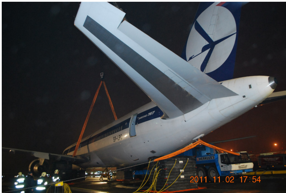
Photo 10. SP-LPC airplane plane lifted up by crane and airbags.
