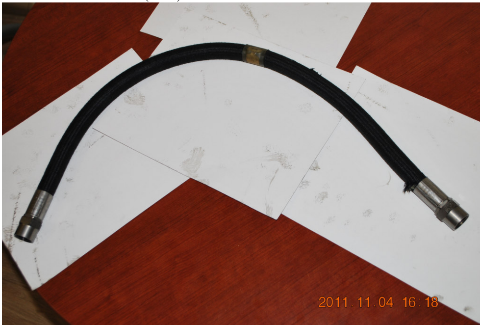
Photo13. Damaged hydraulic hose of the landing gear extension system of SP-LPC airplane.
