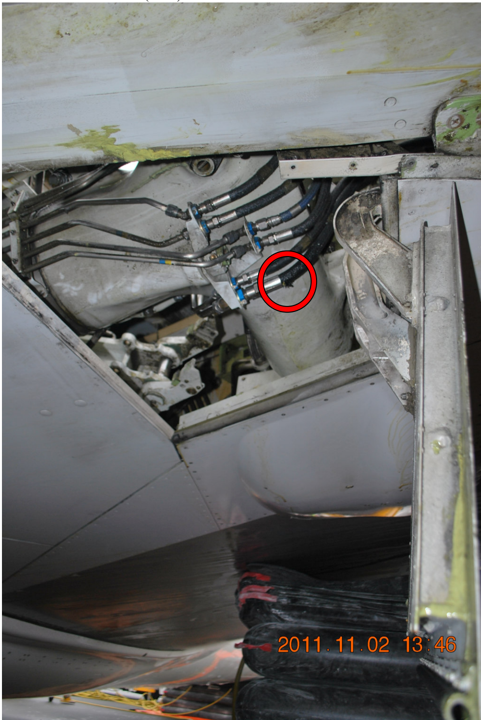
Photo 7. View of the hydraulic hoses of the right main landing gear of SP-LPC airplane
