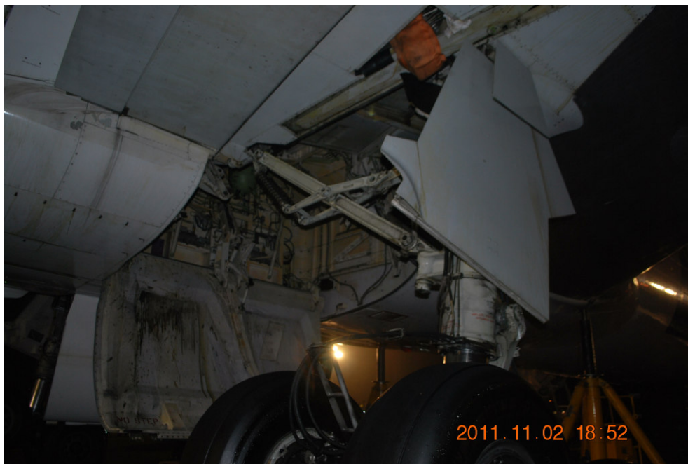
Photo 11. Extended right main landing gear after lifting SP-LPC airplane.
