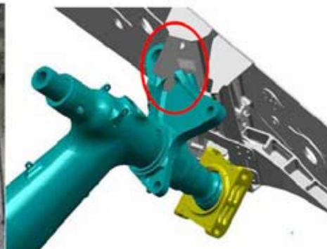
3. Shock Strut / Retract Arm Jams on and destroys upper part of inboard Trunnion Support Fitting
