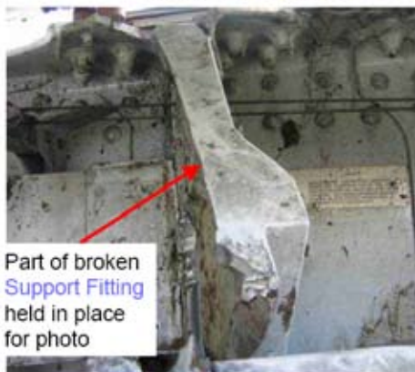
3. Shock Strut / Retract Arm Jams on and destroys upper part of inboard Trunnion Support Fitting
