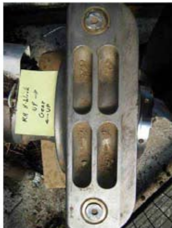
1. Initial Impact Forward Trunnion fused
